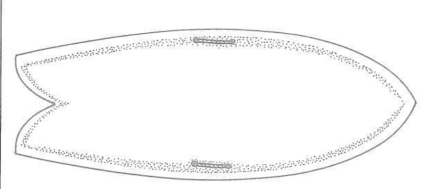
Length: 56" or 61" Width: 20-1/4" Bottom: Flat, w/nose to tail rocker Rails: Down rounded Fin System: Fins Unlimited short box, 4-1/2" custom fiberglass fins.
